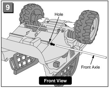
• Slide the front axle (longest) through the holes in the front end of the vehicle body.
